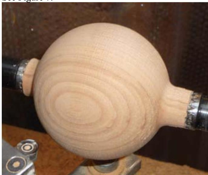
**Figure 7. The ball is now turned as far as it can go when mounted between centers.**
